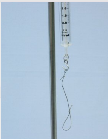
Fishing line on the power gauge hangers
