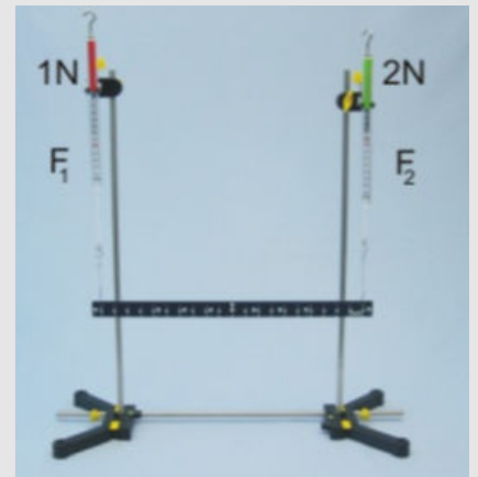
Measuring the forces F_1 and F_2
