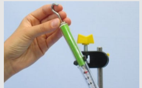
Inserting and adjusting the force gauges
